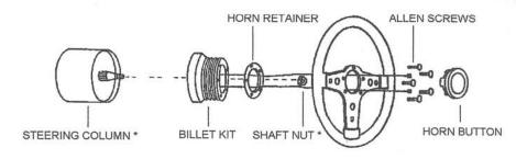
ATTN: THE HUB IN THIS KIT IS DESIGNED TO FIT TIGHTLY ON THE SHAFT AND TO BE DRAWN DOWN BY TIGHTENING THE SHAFT NUT.
