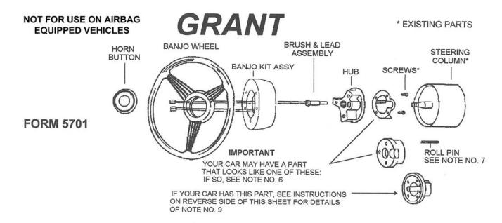
This GRANT Banjo Wheel Kit can only be used on a GRANT Banjo Wheel and is not for use on any other type of wheel or a competitor's product. It cannot be used in conjunction with our Vehicle Security System.
